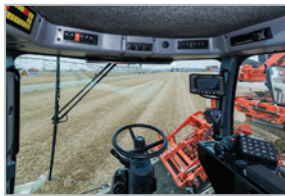
Cab rotates 90° into harvesting position for excellent visibility and operator comfort
