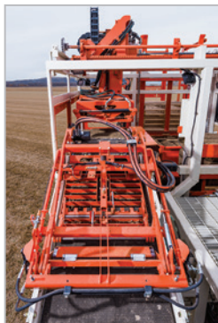
Powered roll-up, automatic flap control system
