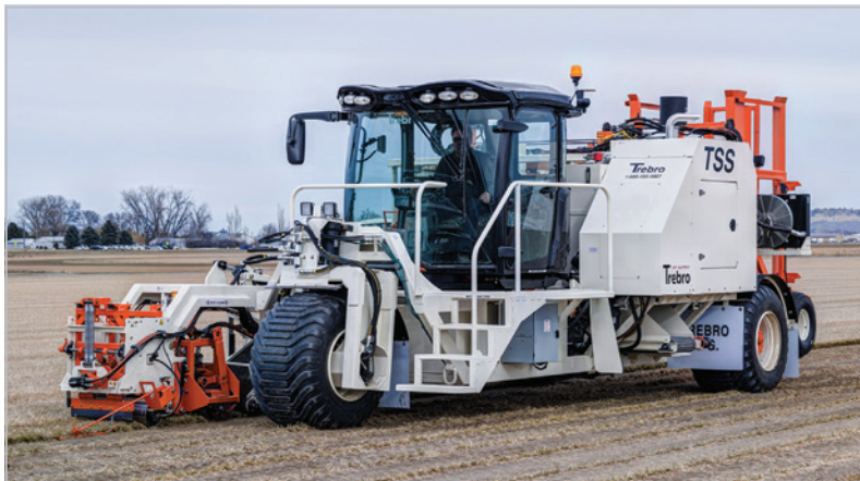
Cross-conveyor scrap dump puts scrap out of the way
