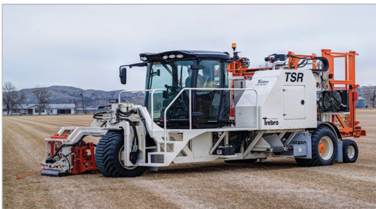
Powered roll-up, automatic flap control system
